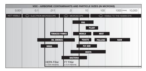
All SmartVent systems feature high grade F7 filters\* that capture up to 90% of 0.4 microns particles such as fine pollens, dusts and allergen from the air making the air cleaner to breathe. High quality HEPA filters are also available for asthma and allergy sufferers.
